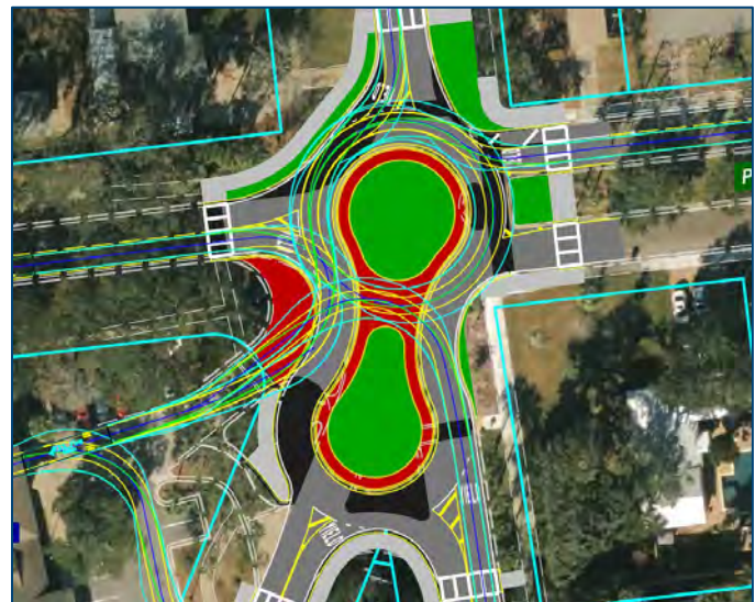
Vehicle movements through the roundabout are simulated using AutoTURN (source: FDOT)
